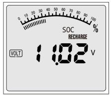
SOC: State of Charge VOLT: Battery Voltage
