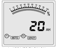
CAR BATTERY TYPE: select the testing standard(CCA,IEC,EN,DIN,CA) MOTO BATTERY TYPE: select the correct battery capacity(AH)
